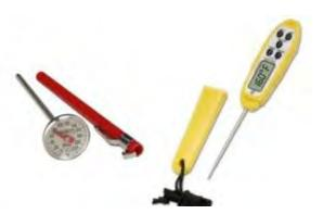
Instant Read Thermometer – analog models are durable, safe, and cheap but they take 15 seconds or more to read the temperature and they require calibration (buy placing in ice water or boiling water then turning the nut on the back of the thermometer) a few times a year, digital models are quick and effective and require you to change the battery every year or two but cost more and are prone to breakage.
